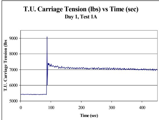
**Figure 4 Day 1, Test 1A, The tension on the takeup carriage stabilizes at approximately 7,000 lbs.**
