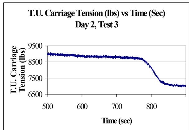
**Figure 6 The running tension of the conveyor has now increased to approximately 9,000 lbs. without load. Similarly, the tension begins to decrease as load is transferred onto the conveyor.**
