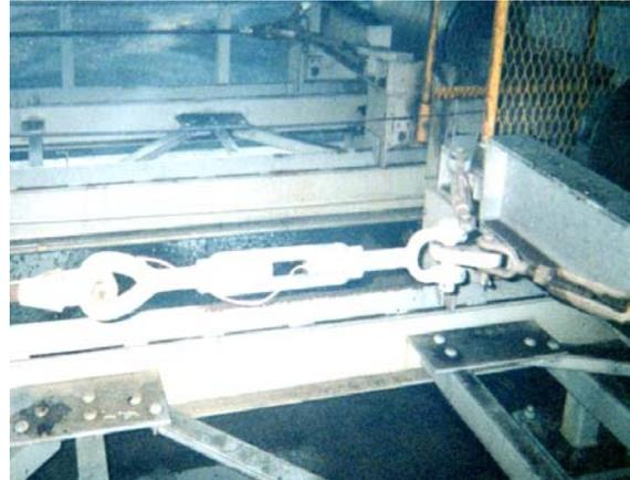
**Figure 3 Internally gauged turnbuckle attached to the takeup carriage.**
