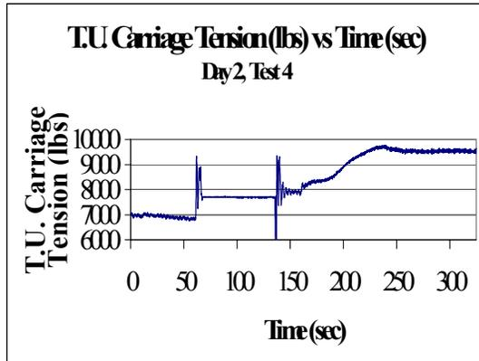
**Figure 7 The conveyor is moving coal at 600 tons/hour and is shut down under load approximately one minute into the test. The material load is removed from the belt directly after the conveyor is restarted. The tension on the takeup carriage increases to approximately 9,700 lbs.**
