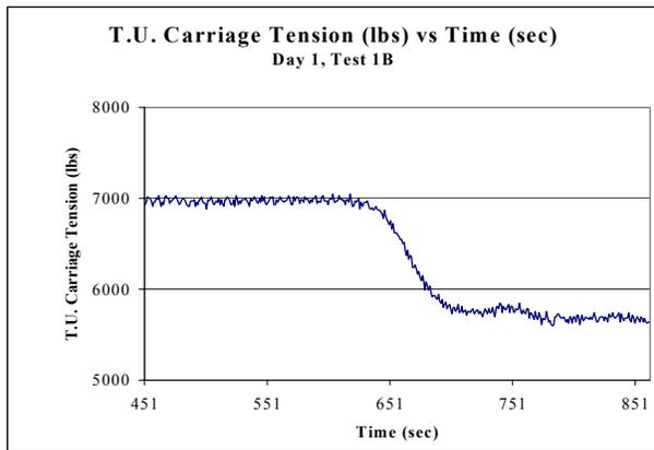
**Figure 5 Day 1, Test 1B, The tension on the carriage decreases as material is loaded on the belt.**
