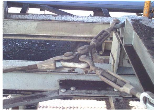
**Figure 2 Wire rope attached to the takeup carriage.**
