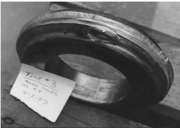
**Figure 3** Hub portion of a fatigue sample after testing to failure. Failure initiated at toe of cruciform weld and propagated around weld circumference and through end disc plate.
