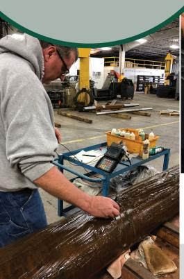
Note: If rim shell materials are stainless-steel the ultrasonic inspection may be replaced with radiography and magnetic particle inspection replaced with liquid dye penetrant inspection.
