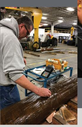
Note: If rim shell materials are stainless-steel the ultrasonic inspection may be replaced with radiography and magnetic particle inspection replaced with liquid dye penetrant inspection.
