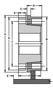
QD® has a primary benefit of bushing interchangeability with other shaft mounted components. Its shallow taper provides a high mechanical advantage to assure dependable clamping to the shaft.
