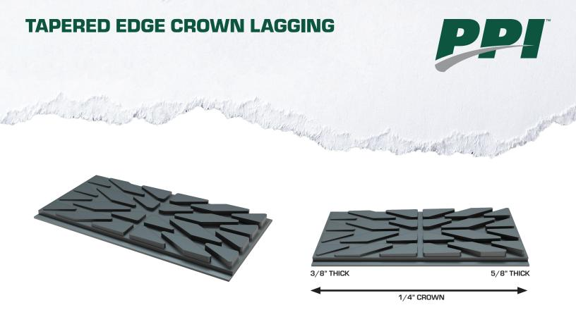
PPI's Tapered Edge Crown Lagging provides a smooth transition from full lagging thickness as it tapers down providing a 1/4" of crown over the span of 10". This gradual taper provides a belt-friendly crown in the face of the pulley, keeping the belt centered. The scalloped backer plate allows the product to be field formable to fit a wide range of pulley diameters.
