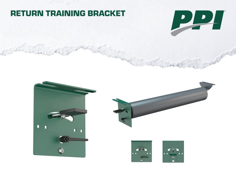
Tracking a conveyor belt has long been a challenge in the bulk material conveying industry. One of the most effective ways of manipulating belt tracking is by knocking idler rolls. PPI's patented Return Training Bracket allows site personnel to knock or skew return idler rolls with ease. PPI's innovative design allows the user to fine tune the return roll position achieving optimal belt travel.
