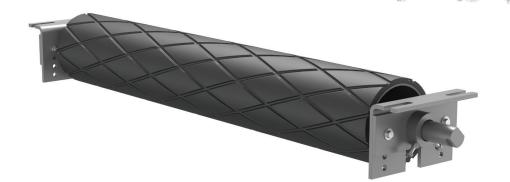
The PPI Pro Tracker is a great solution for your belt tracking issues. With continuous engagement on the return belt, this lagged trainer pivots to guide the belt to its central position resulting in less material loss and belt damage. Mounted with two adjustable brackets for easy installation and no exposed frame for material build up, the PPI Pro Tracker will become your most reliable belt tracking idler.
