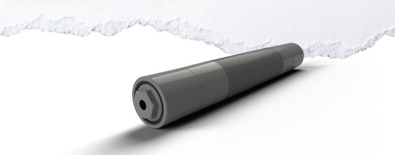
PPI has designed a new Tight Transfer Roller (TTR) for high load unit handling applications. The TTR utilizes a patented cartridge design to maximize the load capacity while minimizing diameter. The 2.25" roller diameter is ideal for conveying applications requiring minimum gap to reduce package movement on belts operating in excess of 540 feet per minute. The TTR roller has been shown to provide longer bearing life than through-shaft ball and spherical roller bearing designs.
