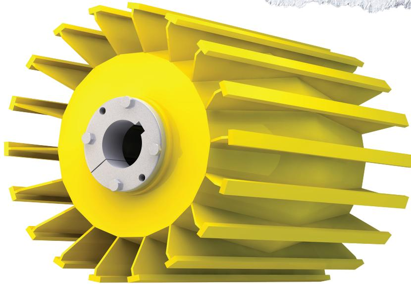
The Quarry Max Duty Wing pulley is made for severe applications where wing folding and abrasion issues are a concern. It resists wing folding by utilizing an end disc when necessary to keep wing heights ideal, short enough to resist folding, long enough to provide adequate rigidity. Ideally suited for harsh applications and for very abrasive conditions.
