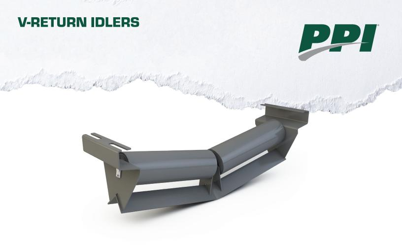
PPI's V-Return Idlers are available with 4.5" and 7" drop heights and are built with a 10° two roll trough configuration that allows gravity to naturally keep the belt centered. The shorter two roll design enables the user to implement much lighter rolls than the traditional single roll configurations.
