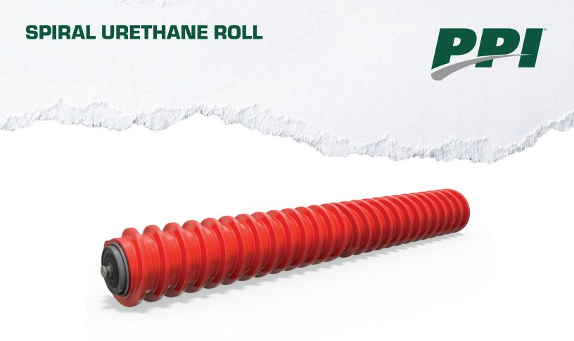
Spiral Urethane Rolls provide an ever changing point of contact on the conveyor belt surface allowing cleaning action without beating the belt. The spiral design is made out of urethane which promotes extended wear qualities and abrasion resistance.
