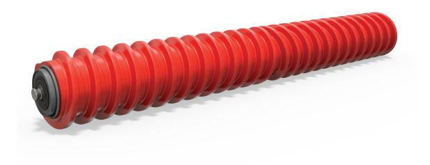
PPI's Spiral Urethane Rolls provide an ever changing point of contact on the belt surface that allows cleaning action without beating the belt. The spiral design is made out of urethane which promotes extended wear qualities and abrasion resistance.
