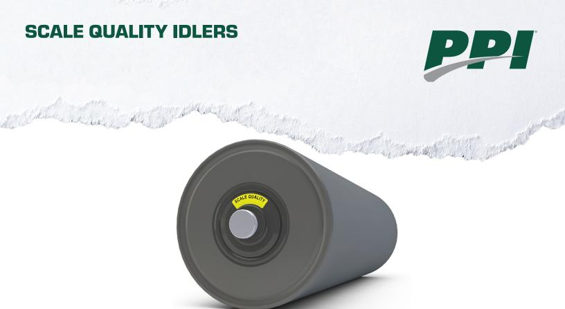
In weighing applications accuracy is vital, so a smooth rotating idler roll is a key component in any weigh scale system. At PPI, the tube of each scale quality idler is manufactured to ensure TIR (Total Indicator Runout) is within .015". After the manufacturing process is complete each roll is measured confirming tolerances have been met and then the roll is clearly marked scale quality.
