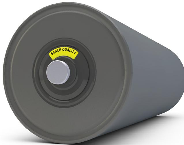
In weighing applications accuracy is vital, so a smooth rotating idler roll is a key component in any weigh scale system. At PPI, the tube of each scale quality idler is manufactured to ensure TIR (Total Indicator Runout) is within .015". After the manufacturing process is complete each roll is measured confirming tolerances have been met and then the roll is clearly marked scale quality.
