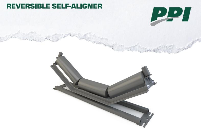
Traditional guide arm self-aligners will not function properly in reversing belt applications due to the guide arms being belt direction sensitive. PPI's Reversible Self-Aligner is equipped with either a slider plate style or a guide roller version, both configurations operate under the same principle, as the belt wanders off of centerline it engages the actuators causing the trainer to steer the belt back to center.
