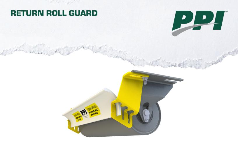
The PPI Return Roll Guard provides a barricade at the pinch point created by the belt passing over a return roll. The 1 1/2" or 4 1/2" mounting brackets provide easy installation on 4", 5" or 6" rolls utilizing the return bracket's mounting bolts. While normally used on return rolls with seven feet or less vertical clearance from the ground or decking, it may be used on any return roll.
