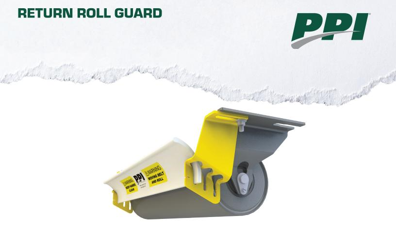
The PPI Return Roll Guard provides a barricade at the pinch point created by the belt passing over a return roll. The  $1\,1/2$ " or  $4\,1/2$ " mounting brackets provide easy installation on 4", 5" or 6" rolls utilizing the return bracket's mounting bolts. While normally used on return rolls with seven feet or less vertical clearance from the ground or decking, it may be used on any return roll.
