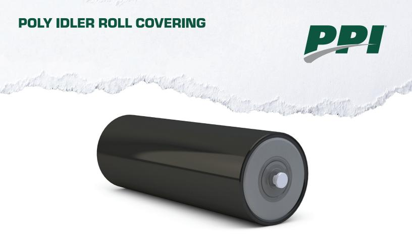
Obtain the material shedding characteristics of a polymer roll with the proven reliability of PPI's standard steel roll. Wear life is extended by pressing a plastic sleeve over the shell of the idler roll. In many applications, the plastic surface of the roll sheds wet sticky material that otherwise may build up on a standard steel roll.
