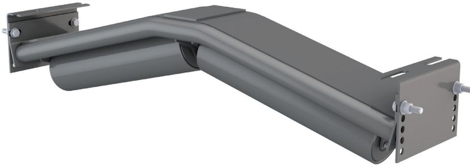
Inverted V-Return (IVR) Idlers are used to positively track the belt on the return side of the conveyor. The PPI IVR is adjustable to increase the displacement and the resulting tracking force on the belt.
