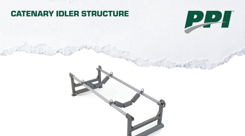
PPI catenary structures incorporate a user friendly design allowing for ease of assembly and tear down while letting the operator reconfigure their conveyor as the mining process dictates. Floor stands equipped with chain-slot brackets allow roof or floor mount configurations based on specific terrain at the mine. Available in CEMA C, D, and E for 24" - 72" belt widths. For wider belts please contact your sales representative for assistance.
