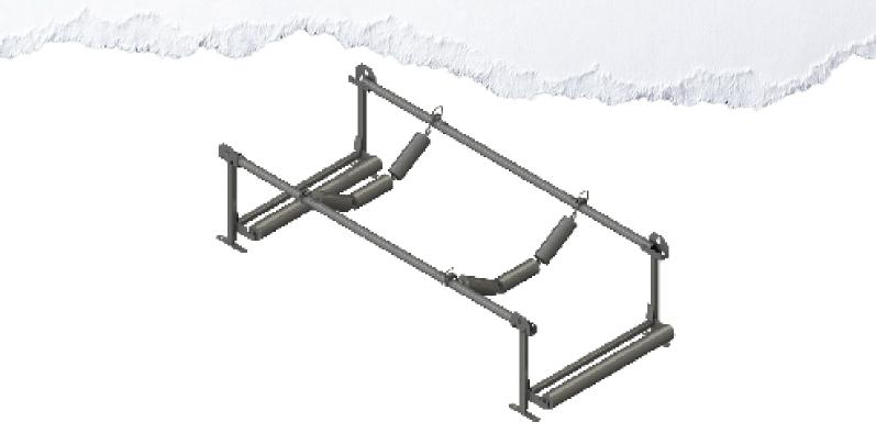
PPI catenary structures incorporate a user friendly design allowing for ease of assembly and tear down while letting the operator reconfigure their conveyor as the mining process dictates. Floor stands equipped with chain-slot brackets allow roof or floor mount configurations based on specific terrain at the mine. Available in CEMA C, D, and E for 24" - 72" belt widths. For wider belts please contact your sales representative for assistance.
