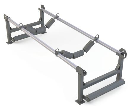
PPI catenary structure incorporates a user friendly design that allows easy assembly and tear down that lets the operator reconfigure their conveyor as the mining process dictates. Floor stands equipped with chain-slot brackets allow roof or floor mount configurations based on specific terrain at the mine. Available in CEMA C, D, and E for 24" - 60" belt widths. For wider belts please call for application assistance.
