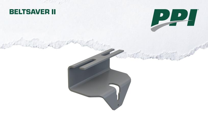
Protecting the most valuable piece of the conveyor system, the belt, is vital to maintenance personnel. PPI's Beltsaver bracket outward bend design allows the belt to track off of the centerline further than traditional style return roll drop brackets. The extra space provided by these drop brackets alleviates damage to the belt and minimizes the risk of the belt cutting through drop brackets.
