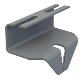
Protecting the most valuable piece of the conveyor system, the belt, is vital to maintenance personnel. PPI's Beltsaver Bracket outward bend design allows the belt to track off of the centerline further than traditional style return roll drop brackets. The extra space provided by these drop brackets alleviates damage to the belt and minimizes the risk of the belt cutting through drop brackets.
