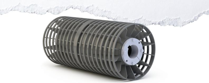
The PPI Spiral Wing and Spiral Plus Wing pulleys are formed by winding flat bar spirally from the center of a wing pulley to the outside ends. This continuous belt contact design eliminates excessive noise and vibration, while still providing a cleaning effect and allowing a path for debris to escape rather than being trapped between the pulley and belt.
