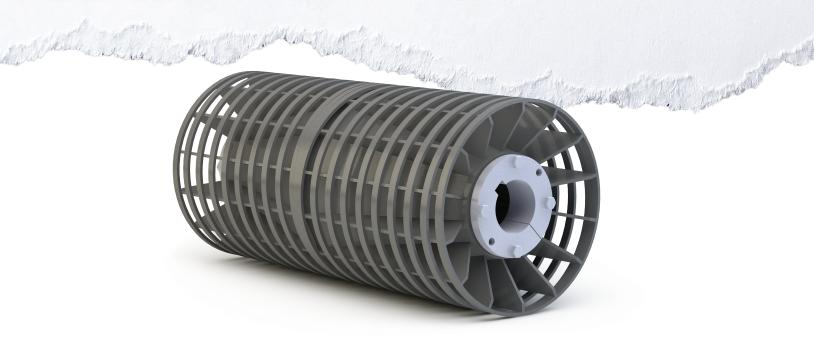
The PPI Spiral Wing and Spiral Plus Wing pulleys are formed by winding flat bar spirally from the center of a wing pulley to the outside ends. This continuous belt contact design eliminates excessive noise and vibration, while still providing a cleaning effect and allowing a path for debris to escape rather than being trapped between the pulley and belt.
