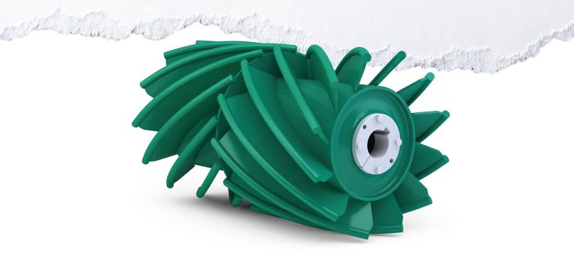
The PPI Bar Constructed Herringbone Wing was designed for those applications where conventional wings suffer from excessive material lodging and wing folding. The extreme wing angles of up to 45°, use the pulleys rotation to eject material out the sides of the pulley rather than recirculating it as a conventional wing often does. These extreme angles and optimized wing height, along with a center reinforcement disc, all combine to make an incredibly strong design that excels where others fail.
