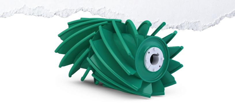
The PPI Herringbone Wing was designed for those applications where conventional wings suffer from excessive material lodging and wing folding. The extreme wing angles of up to 45°, use the pulleys rotation to eject material out the sides of the pulley rather than recirculating it as a conventional wing often does. These extreme angles and optimized wing height, along with a center reinforcement disc, all combine to make an incredibly strong design that excels where others fail.
