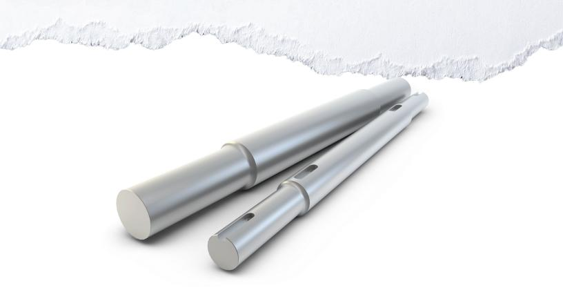
PPI conveyor pulley shafting is a vital part of the total pulley assembly. Standard PPI shafting is AISI 1045. The higher carbon content in a AISI 1045 results in a very strong steel that machines to a smooth finish. Normally, PPI uses T&P for shafting up through 5-15/16". While, hot rolled and; or forged shafting (depending upon size, availability, and specifications) is used above a 6" diameter.
