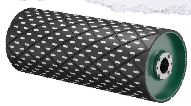
PPI's patented VEC Lagging starts with SBR or Neoprene lagging that is hot vulcanized onto a pulley. Our uniquely designed tiles are then embedded in the vulcanized lagging. This design eliminates seams, where failures often start. It also allows ceramic lagging to be applied to pulleys as small as 4" in diameter, something that cannot be achieved using cured lagging pads.
