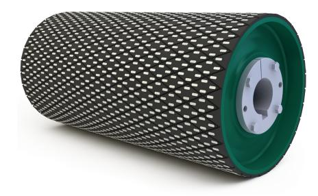
PPI's patented VEC Lagging starts with SBR or Neoprene lagging that is hot vulcanized onto a pulley. Our uniquely designed tiles are then embedded in the vulcanized lagging. This design eliminates seams, where failures often start. It also allows ceramic lagging to be applied to pulleys as small as 4" in diameter, something that cannot be achieved using cured lagging pads.
