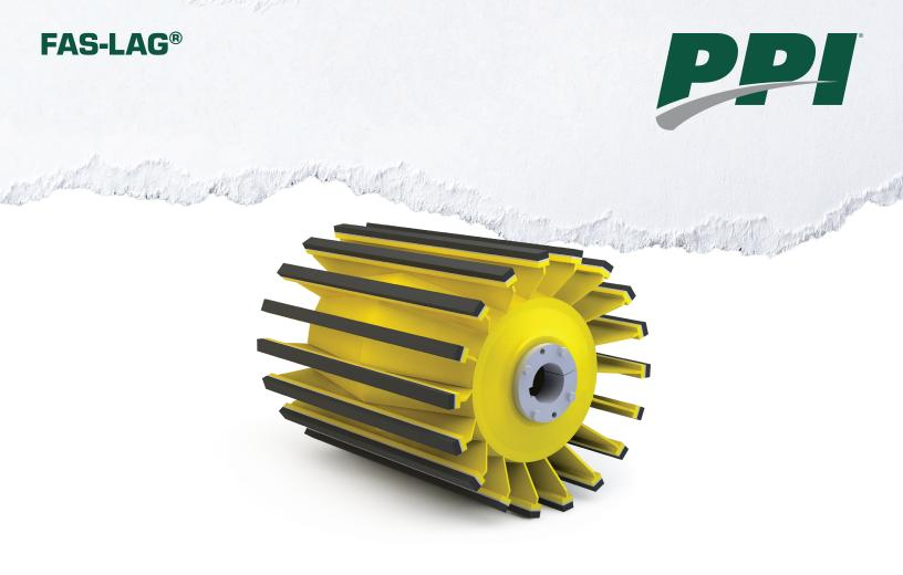
Fas-Lag® is an easy to install wing pulley lagging system designed to be welded to a wing pulley's flat contact bar to provide additional traction with the belt and added protection for the contact bar. It may also be used to lessen material buildup on contact bars and reduces impact and wear on mechanical belt splices.
