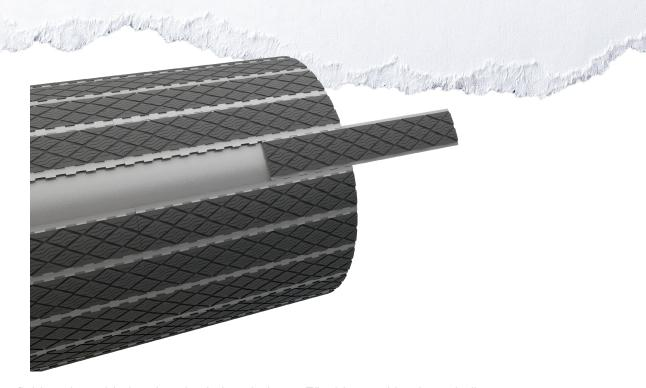
$\mathsf{EZ}\text{-}\mathsf{LAG}^\mathsf{TM}$  is a field replaceable lagging that's bonded to a 5" wide steel backer, similar to Craft-Lag<sup>®</sup>. However, unlike Craft Lag,  $\mathsf{EZ}\text{-}\mathsf{LAG}$  has perforations in the steel backer that allow it to be formed to fit any pulley diameter 12" and over.
