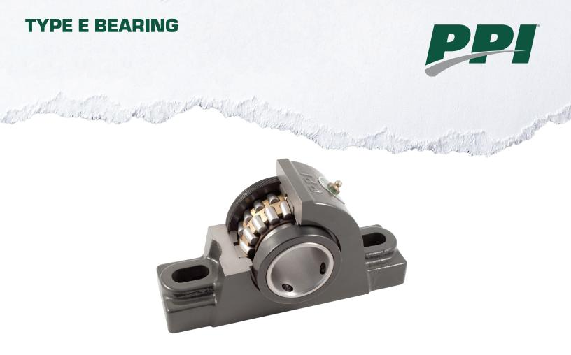
The PPI Type E pillow block bearing was designed specifically for the challenges of multiple conveyor applications. That's why our Type E bearing utilizes a double row spherical bearing that makes a misalignment of  $\pm$  2 degrees possible. This allows the bearing to be more forgiving of mounting positions that are less than perfect. Additionally, a double lip nitrile contact seal provides the necessary protection from the heavily contaminated applications, common to the conveyor industry.
