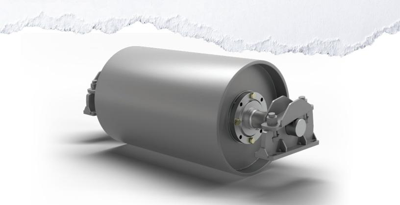
The Static Shaft Pulley (SSP) is a problem solving solution for pulley applications prone to frequent bearing failure. It uses a 22200 series bearing mounted inside the pulley hub to provide exceptional bearing protection. This patented design also uses a taconite sealing system that provides further protection from contaminants entering the bearing.
