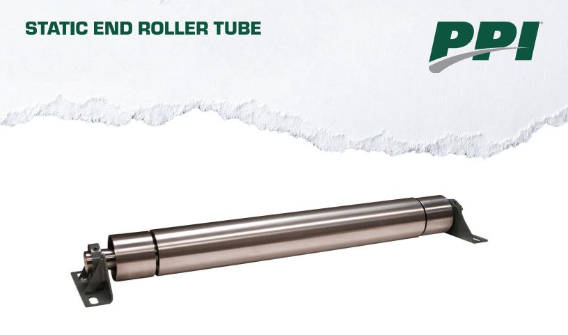
PPI Static End Rollers provide a safe, reliable solution to exposed work zones. They are designed to eliminate the potential pinch point caused between a rotating roller and the moving conveyor belt. Entanglement of Foreign Objects and Debris (FOD) is also reduced as a result of stationary roller ends.
