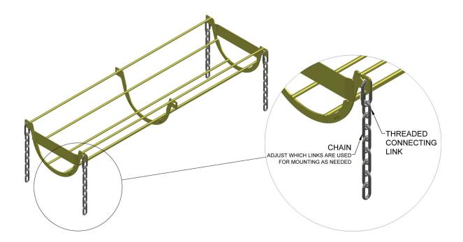
STEP 2 – PPI recommends using bolts to attach the chains to the conveyor structure for added security. Beam clamps are available if requested. If beam clamps are to be used, attach them to each chain. The location to connect them on the chain depends on roll cage mounting location and drop height of the return roll brackets. When mounted, the top of the roll cage should be approximately level with the center of the return roll.
