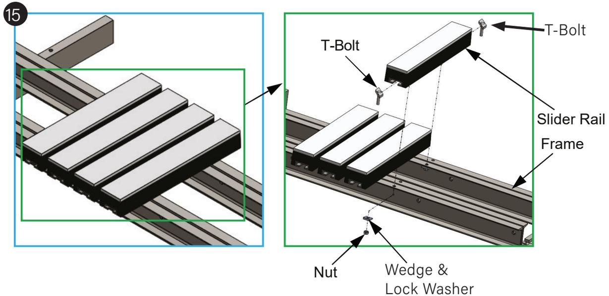
9. Attach the Slider Rails to the frames in the wing positions using the supplied T-Bolts with nuts and washers. Only have the nut snug and do not tighten the nut. The frame positions will need to be adjusted once on the conveyor. See Figure 16.
