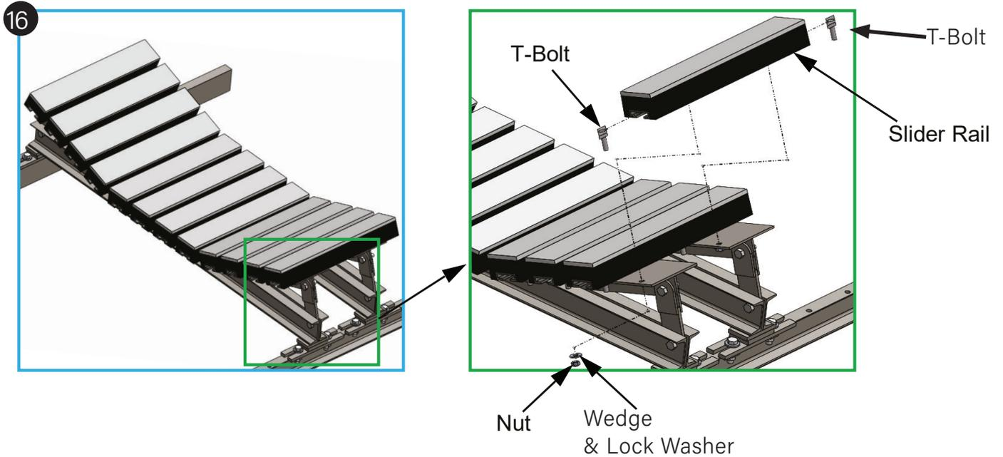
10. Tighten the bolts to secure the frames to the conveyor structure.
