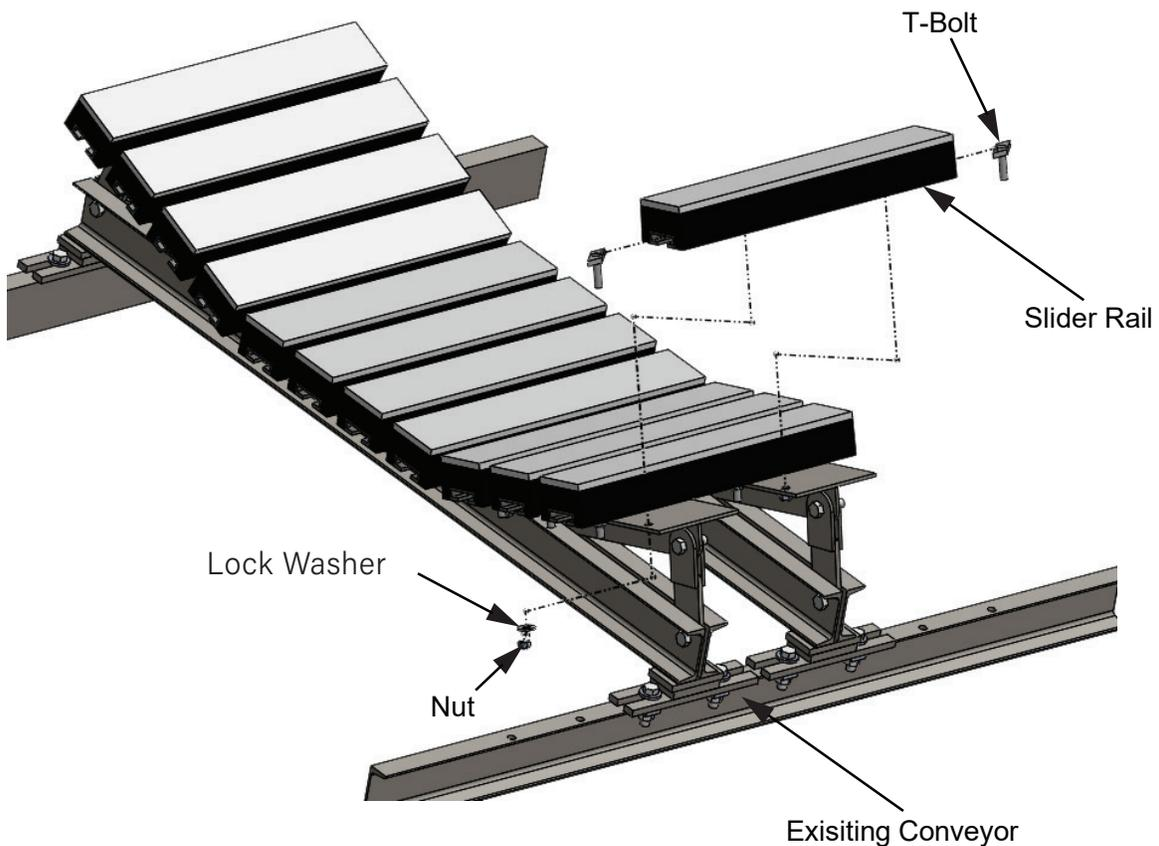
18 SLIDER RAIL BEING REMOVED FROM CENTER POSITION
