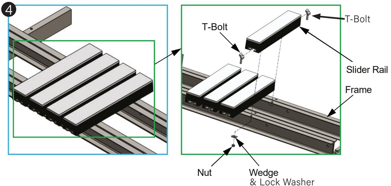
3. Attach the Slider Rails to the frames in the wing positions using the supplied T-Bolts with nuts and washers. Only have the nut snug and do not tighten the nut. The frame positions will need to be adjusted once on the conveyor. See Figure 5.
