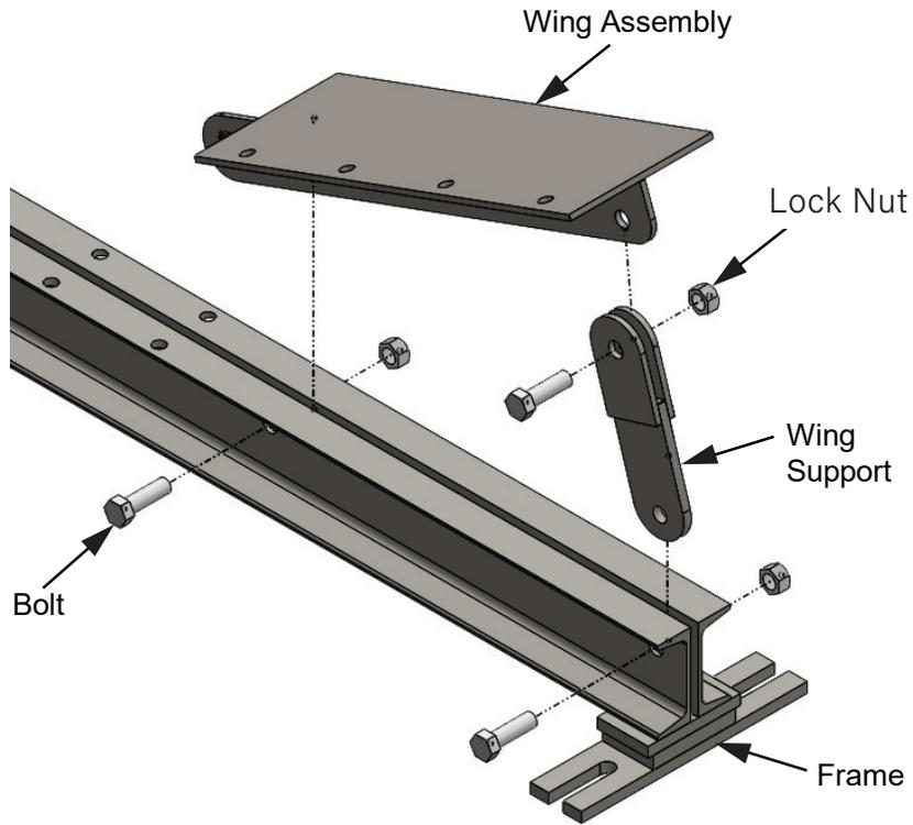
**Wing Support & Wing Assembly Installation:**
