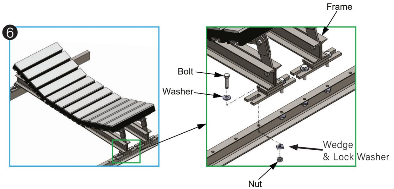
5. Make sure the Impact Bed frames are 90° or perpendicular to the conveyor structure.
