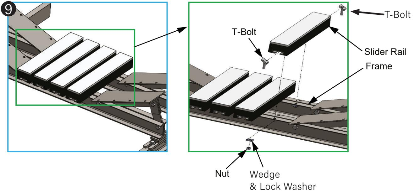
6. Attach the Slider Rails to the frames in the wing positions using the supplied T-Bolts with nuts and washers. Only have the nut snug and do not tighten the nut. The frame positions will need to be adjusted once on the conveyor. See Figure 10.
