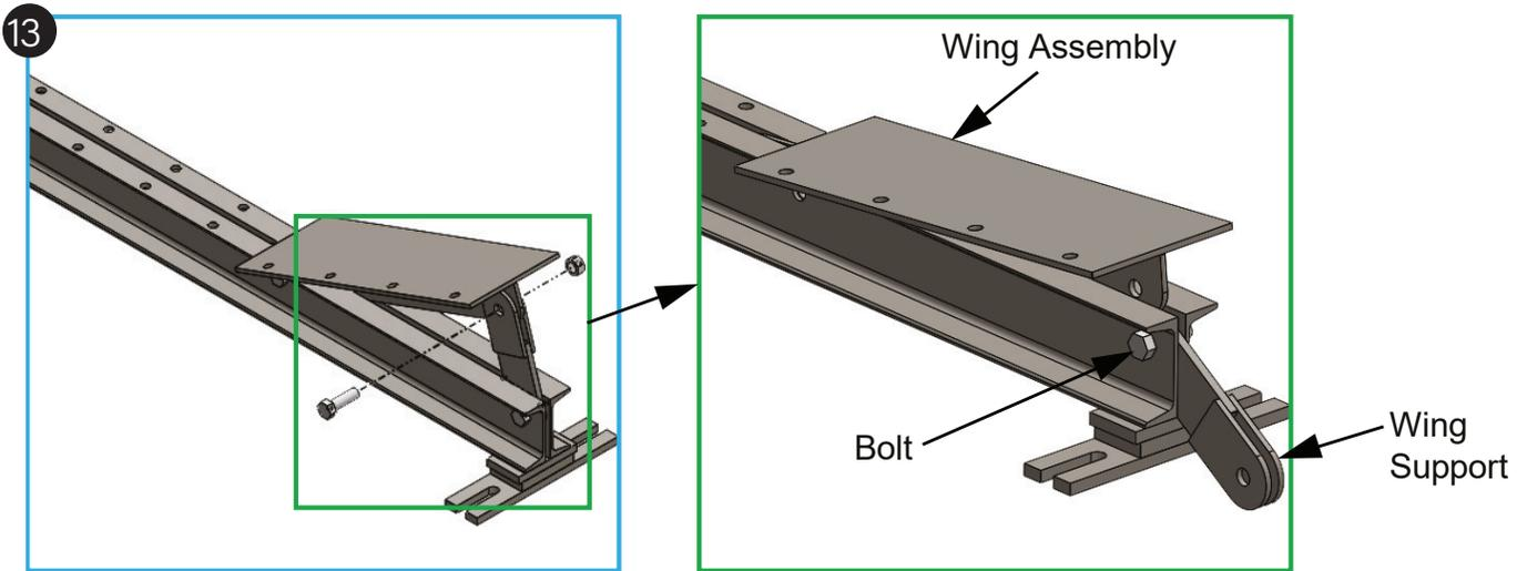
4. For some belt widths the Wing Assembly will need to be removed. To remove the Wing Assembly, remove the remaining bolt in the C-Channel and lift the Wing Assembly off the frame.
