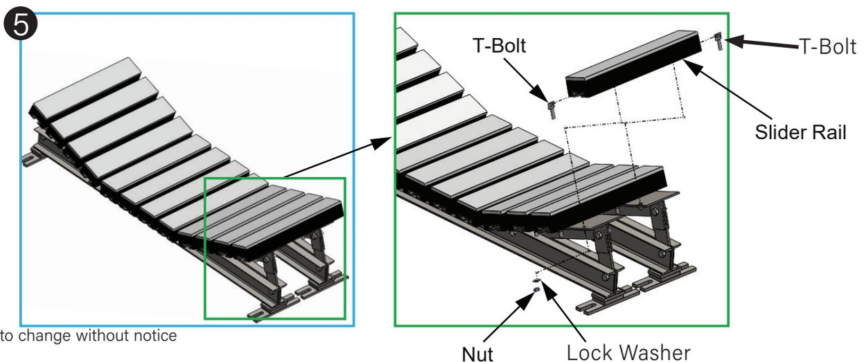
4. Place the fully assembled Impact Bed on the existing conveyor structure as a unit. See Figure 6.
