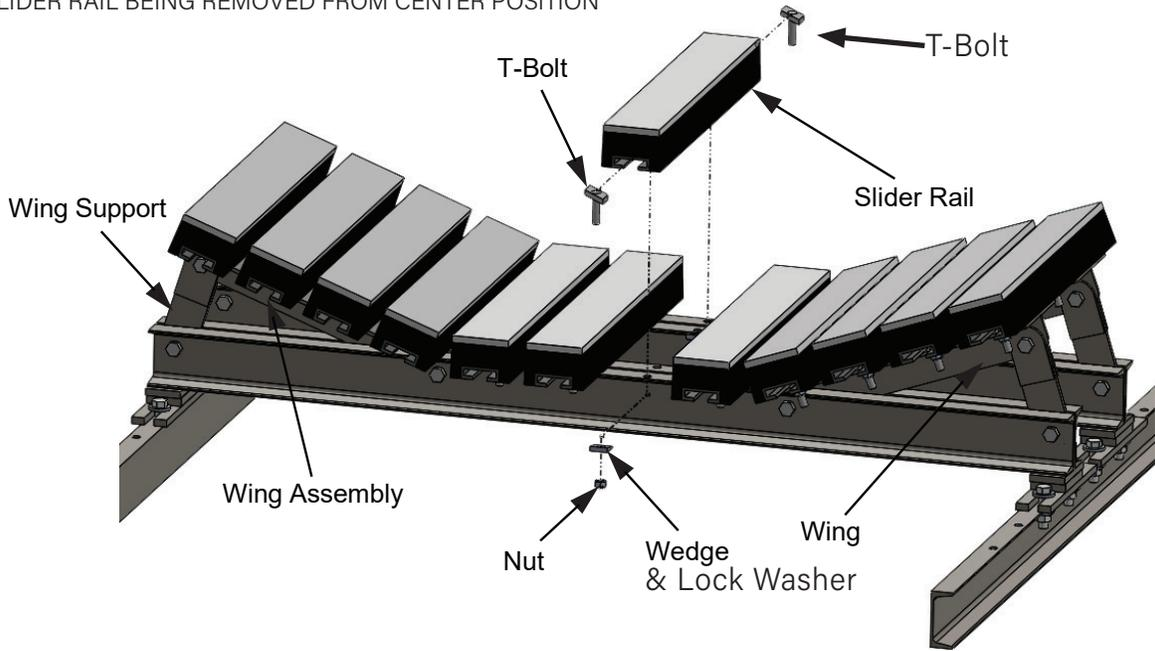
SLIDER RAILS INSTALLATION:
