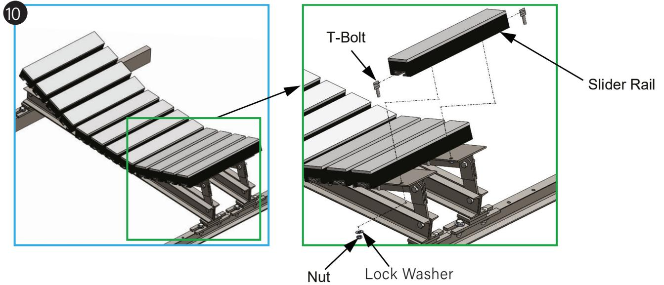
7. Tighten the bolts to secure the frames to the conveyor structure.
