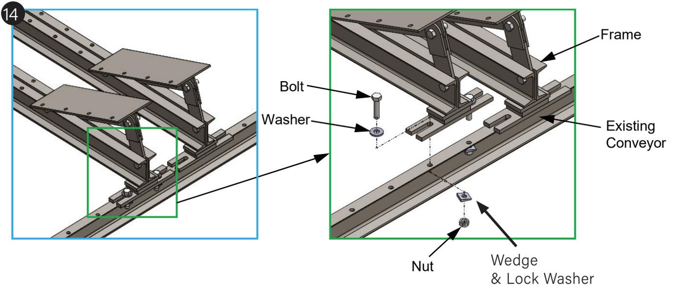
8. Attach the Slider Rails to the frames in the center positions using the supplied T-Bolts with nuts and wedges. Use ONLY one T-Bolt to fasten the Slider Rail to each frame. Each frame consists of 2 C-Channels. The Slider Rail should only be attached to one of the C-Channels in each frame. Only have the nut snug and do not tighten the nut. The frame positions will need to be adjusted once on the conveyor. See Figure 15.
