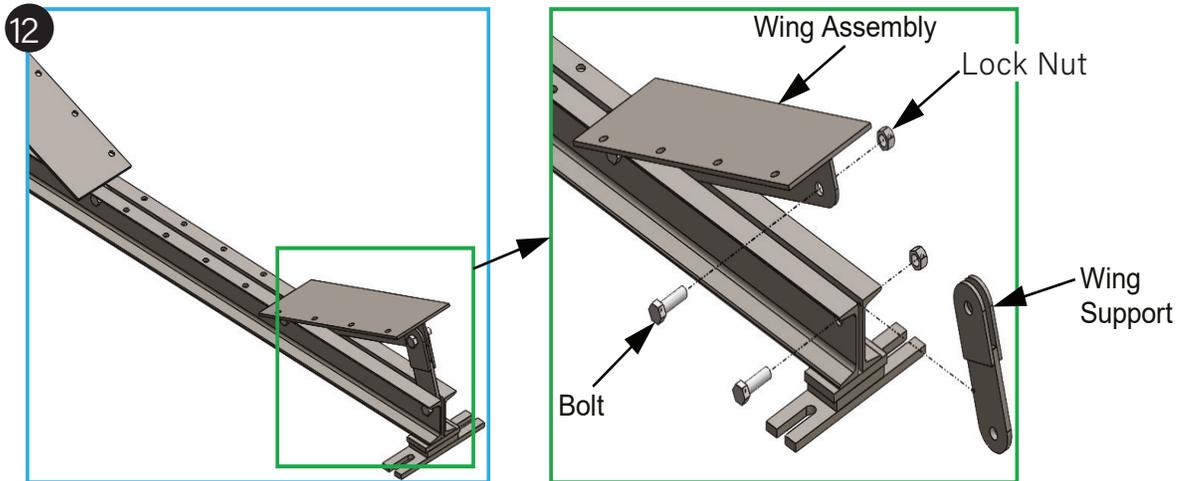
3. For most belt widths the Wing Assembly can be folded flat against the C-Channels of the frame. The bolt connecting the Wing Assembly may have to be loosened. See Figure 13.
