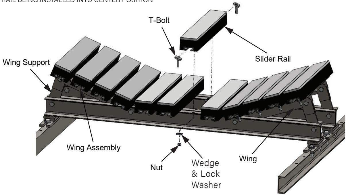
Wing Support & Wing Assembly Removal:
