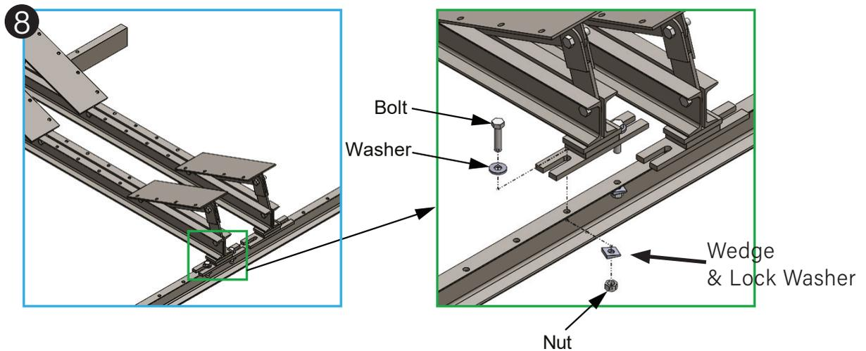
5. Attach the Slider Rails to the frames in the center positions using the supplied T-Bolts with nuts and wedges. Use ONLY one T-Bolt to fasten the Slider Rail to each frame. Each frame consists of 2 C-Channels. The Slider Rail should only be attached to one of the C-Channels in each frame. Only have the nut snug and do not tighten the nut. The frame positions will need to be adjusted once on the conveyor. See Figure 9.
