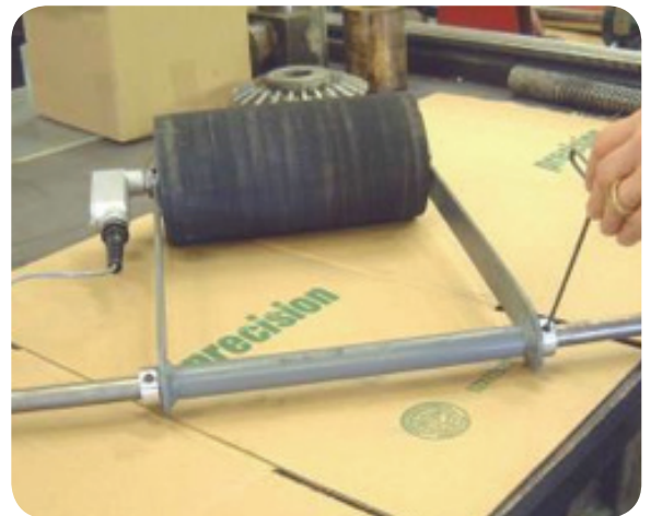
FIGURE 2.3: CSR Mounting Accessories test fit in CSR hinge point. CSR Mounting Accessories sold separately.
