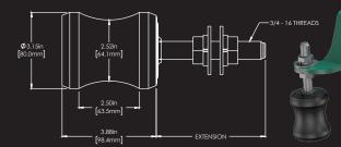
The PPI hourglass guide roll not only helps guide and protect the belt, but it also provides a long-lasting wear life compared to standard steel guide rolls. Made from UV resistant black cast polyurethane, the hourglass guide roll has an exceptional resistance to wear in the most severe conditions.
