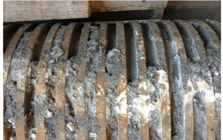
Figure 2 – Spiral Drum plugged with material
