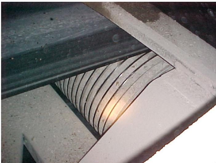
Figure 1 – Spiral Drum plugged with material
