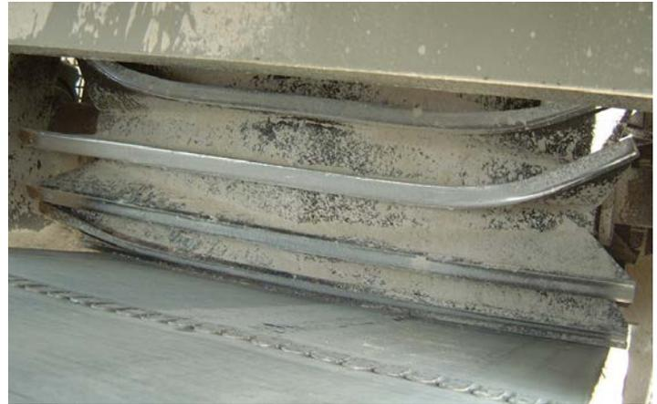
Figure 5 – Tail pulley with bent wings.
