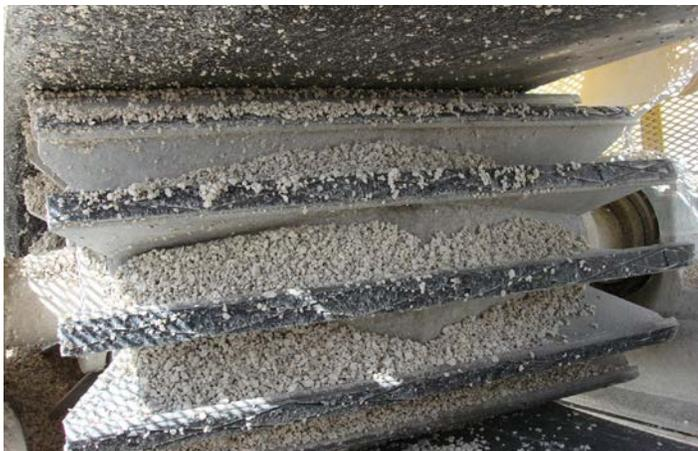
Figure 4 – Wing pulley recycled material.
