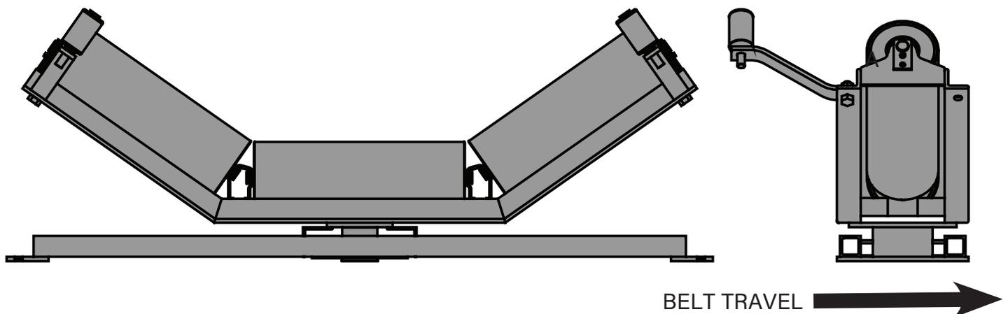
Shifting or tilting of idlers for belt training can be used for belts traveling one direction only. This remedy cannot be used for reversing belt conveyors.
