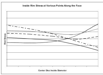
Figure 6 – Inside Rim Stress as a Function of Center Disc Inside Diameter
