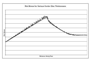
Figure 3 – Rim Stress for Various Center Disc Thickness with 2 CD Development of Center Disc Design Using Finite Element Analysis - SME2012
