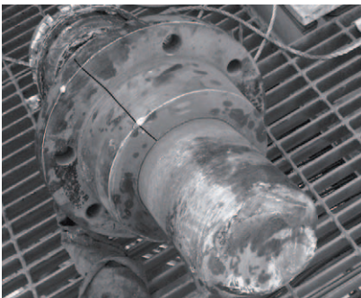
Figure 10. Shaft broken after 3 – 4 months of operation, 13 months after delivery.
