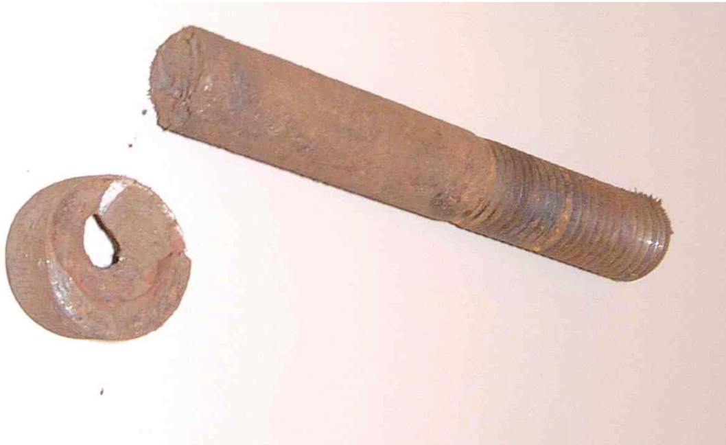
Figure 2: Locking assembly bolt fatigue failure.
