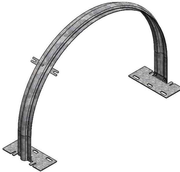
Figure 6: E FULL COVER SUPPORT BAND ASSEMBLY WITH LIST OF COMPONENTS
