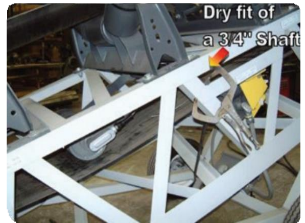
FIGURE 2 .4: Test fit of CSR and Mounting Accessory assembly in conveyor framework, typical both sides.
