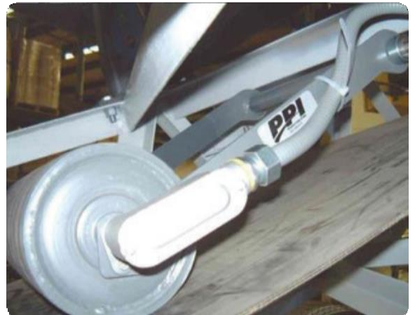
FIGURE 2 .1: Clean Side Return roll in a typical installation. Optional CSR mounting hardware shown. Conduit and wire tire not included.
