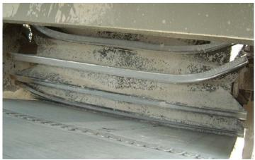
Figure 5 – Tail pulley with bent wings.
