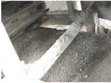
Figure 3 – Wing pulley build up at the tail.
