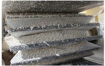
Figure 4 – Wing pulley recycled material.
