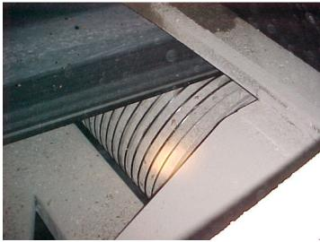
**Figure 1 – Spiral Drum plugged with material** Herringbone Wing – A New Angle on Tail Pulleys - Coal Handling Show 2012
